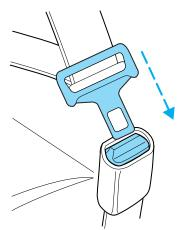
5. To put the retractor in the automatic locking mode, grasp the shoulder portion of the belt and pull downward until all of the belt is pulled out and a click is heard.
